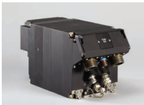
The Rockwell Collins AN/ARC-210 aircraft radio, shown above, is one of the most widely used pieces of avionics in the U.S. military inventory.
