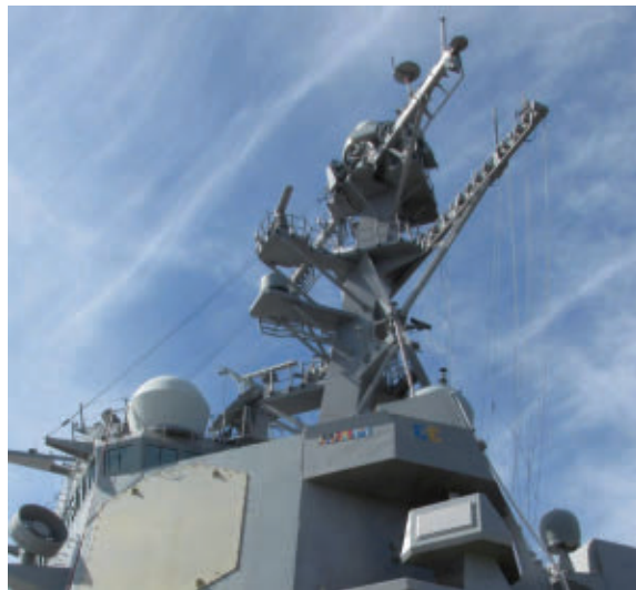
The U.S. Navy is expanding the reach of the shipboard AN/SLQ-32(V)6 Surface Electronic Warfare Improvement Program (SEWIP) Block 2.
