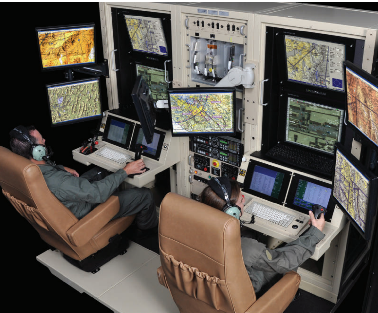
The L-3 Link PMATS is a flight simulator that reproduces the aircrew ground stations of MQ-1 Predator and Predator B/MQ-9 Reaper combat drone pilots and sensor operators.
