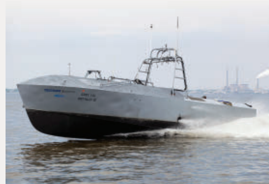
The Textron Common Unmanned Surface Vehicle (CUSV), shown above, is the basis for the U.S. Navy Unmanned Influence Sweep System (UISS).
